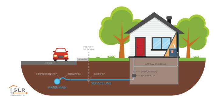
Each service line or connection consists of multiple components. For more information on each component go to <u>www.lslr-collaborative.org/intro-to-lsl-replacement.html</u>
